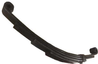
▲ 13072 - Double Eye, Four Leaf Spring- 25 1/4" Long x 1 3/4" Wide 3000# capacity
