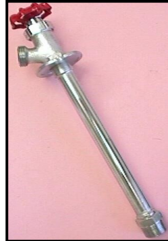
▲ 25538 Frost-Proof Sillcock (3/4" MPT or 1/2" FIP x 8" length) *Silver soldered bottom. 3/4" GHT outlet.
