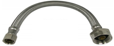
▲ 24313-COMP - 12" Toilet Riser Connection- *3/8" Compression x 7/8" Ball Cock- Stainless Steel- *Use with 039149 Stop Valve (See Page 55)
