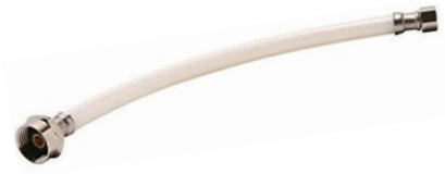
▲ 22313 - 12" Toilet Riser Connection- *1/2" Female Pipe Thread x Ball Cock Thread.
