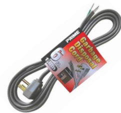
▲ 36215-6 Replacement 6' Length Round Disposal Cord *13 amp- 125 volt. #16 gauge, 3 conductor wire.
