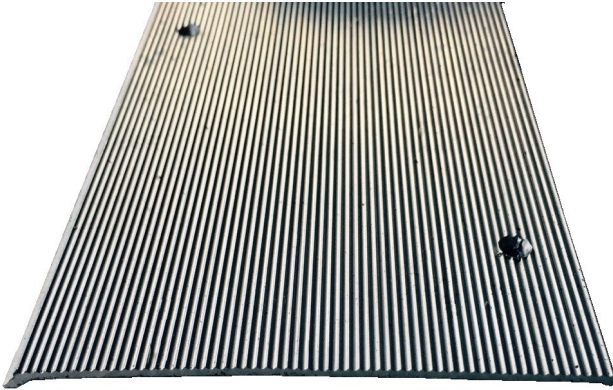
▲ Carpet Seam Binder-Aluminum- Mill Finish Used to bridge seams in separate pieces of carpet. Used with 61085 nails. 61080- 4" x 12" 61078- 2.437" x 12"
